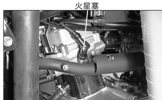
(A) 火星塞間隙0.6~0.7mm
